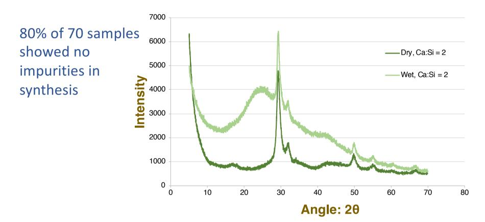
Wet and dry XRD diffractogram of Ca:Si = 2 synthetic C-S-H displaying intrinsic peaks
