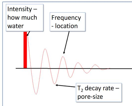
Figure 2: *Excitation pulse and signal decay.*
