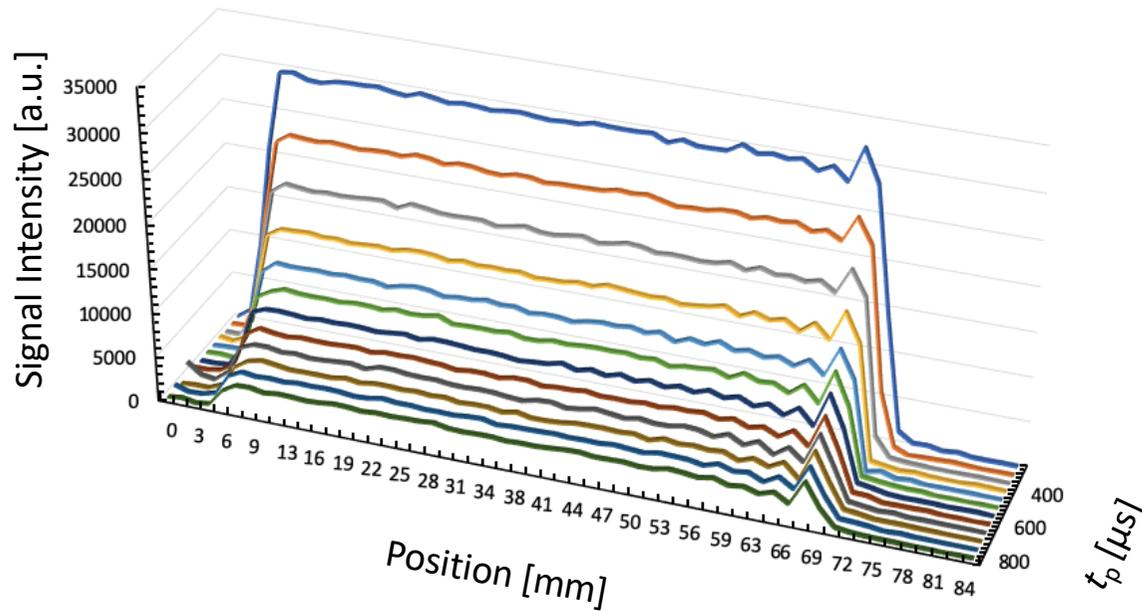
Figure 5 :  $T_2^*$  weighted 1D SPRITE images of the 28-days cured cement paste sample. Twelve profiles are plotted in 50  $\mu\text{s}$  intervals in  $t_p$ , starting from 100  $\mu\text{s}$ . These images represent the moisture present in the cement paste sample ( $w/c=0.4$ ).
