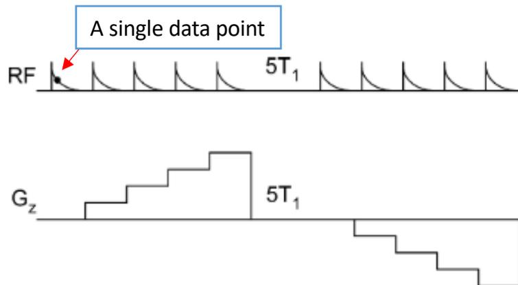
Figure 3: *SPRITE pulse sequence,* K. Deka *et al*, 2006
