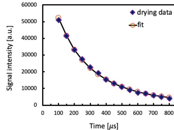
Figure 6: Fitting to the exponential decay to extract  $T_2$  components.
